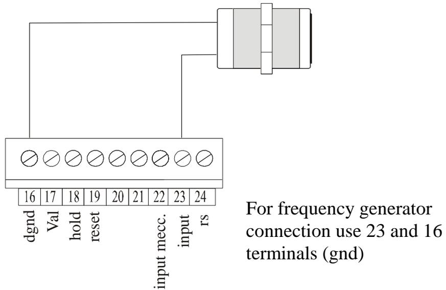
**1.5 WIRING SCHEMATICS FOR TIMER**
