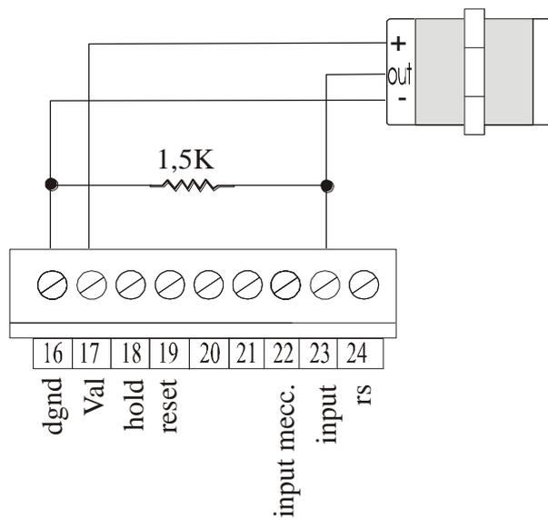
Not amplified MAF 35 sensor connection (maf 35)
