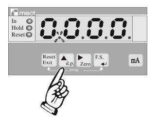
Touch "▲ d.p." key the with the instrument in measuring mode. A decimal point will light up. In order to move this point touch the indicated key until the desired point is reached and than confirm with "FS "
