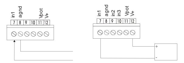
Connection for voltage input (+AD07:60mV) and 3 wire transducer
