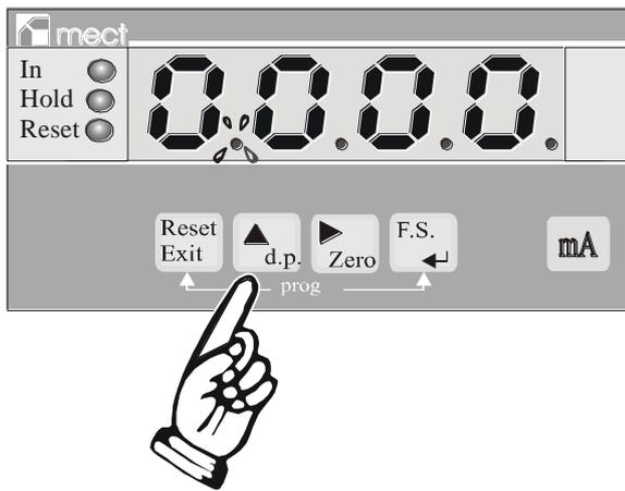
Touch the “ $\blacktriangle$  d.p.” key with the instrument in measuring mode. A decimal point will light up. In order to move this point touch the indicated key until the desired point is reached and then confirm with “FS  $\leftarrow$ ”
