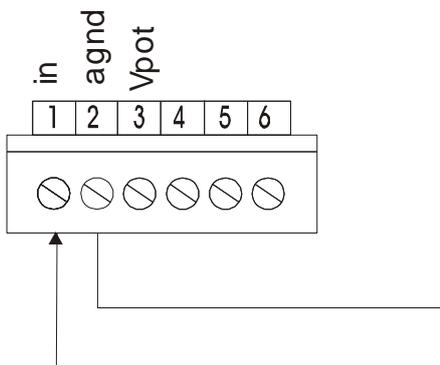
2) Connection for 2 wire transducer with external power supply
